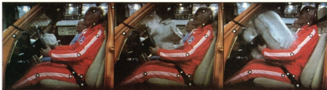
High-speed photography records a test deployment of the Mercedes-Benz Supplemental Restraint System. Within forty-five
